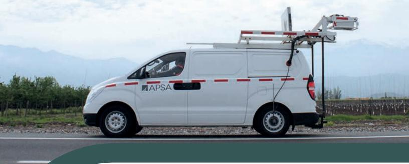
APSA is the first company in Latin America to adapt an automated inspection and processing system for surface deterioration with Laser Crack Measurement System (LCMS), achieving adaptation of the system according to visual inspection methodologies of each country.
